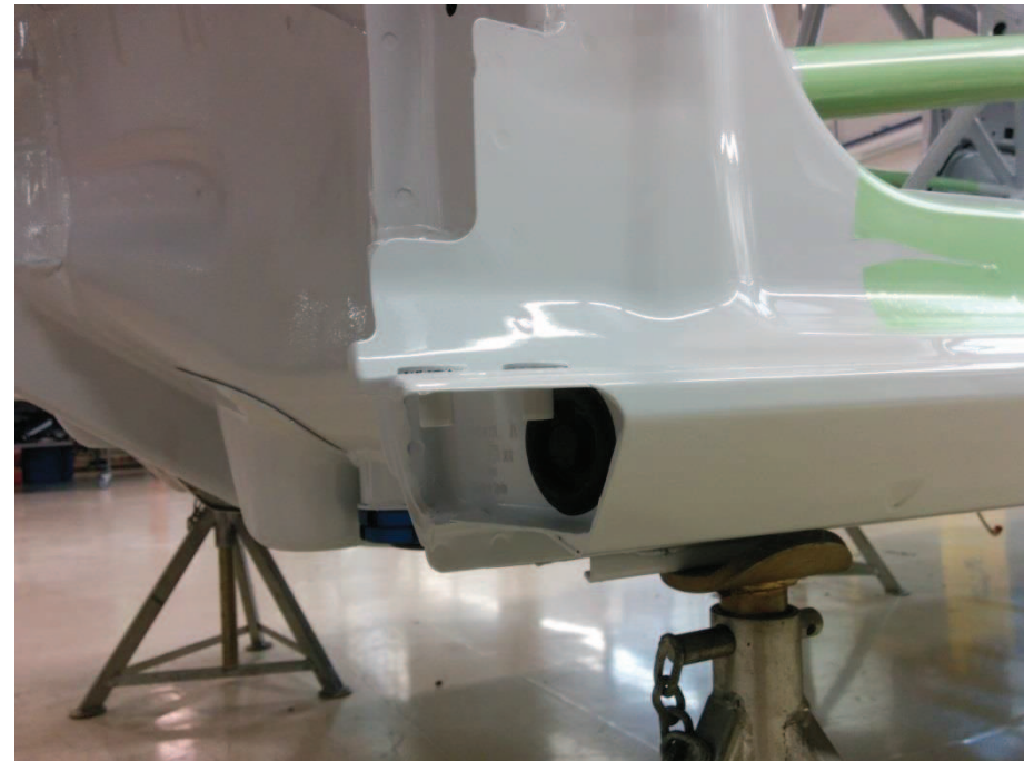
Left side trim cut finished
