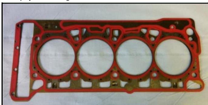
C8-8) Cylinder head gasket from above
