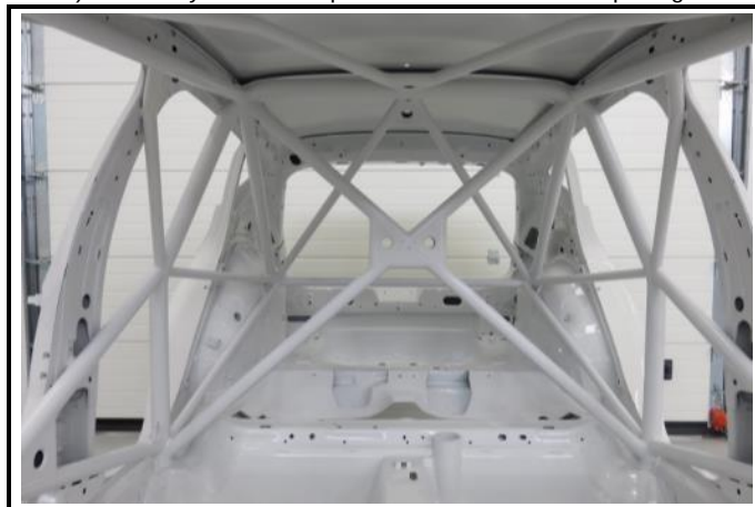
N1-6) Bare bodyshell – Roof seen from cockpit
