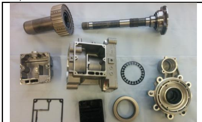
F4-6) Differential dismantled
