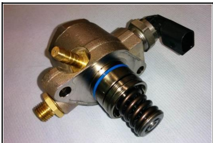
D2-1) High Pressure Fuel Pump - dismounted
