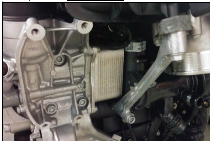
C14-10) Oil cooler – mounted in location
