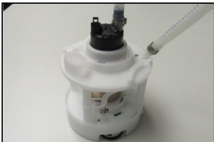
D2-3) Low pressure fuel pump - dismounted
