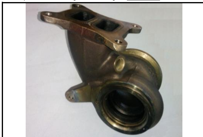
C15-8) Turbine housing of turbocharger - dismounted
