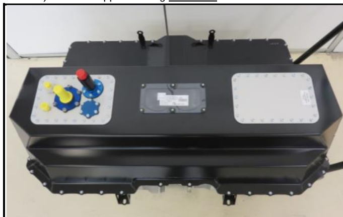
D1- 22) Fuel tank upper housing in location
