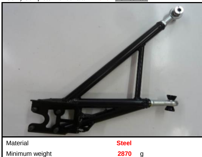
G5-1) Complete wishbone/arm front – dismounted
