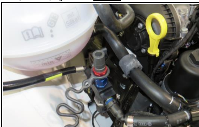
D1-6) Fuel sampling connector in location
