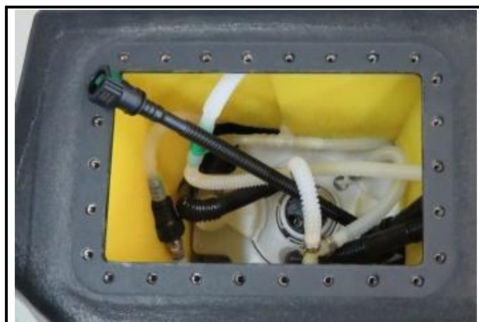
D2-4) Low pressure fuel pump - in location
