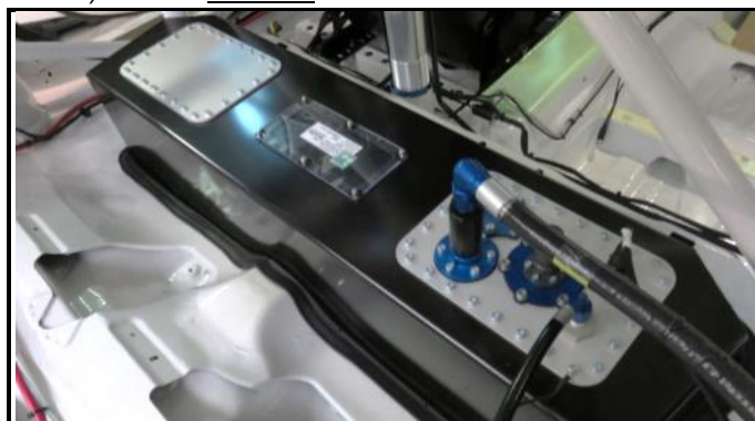
D1- 20) Fuel tank filler cover and fire wall in location
