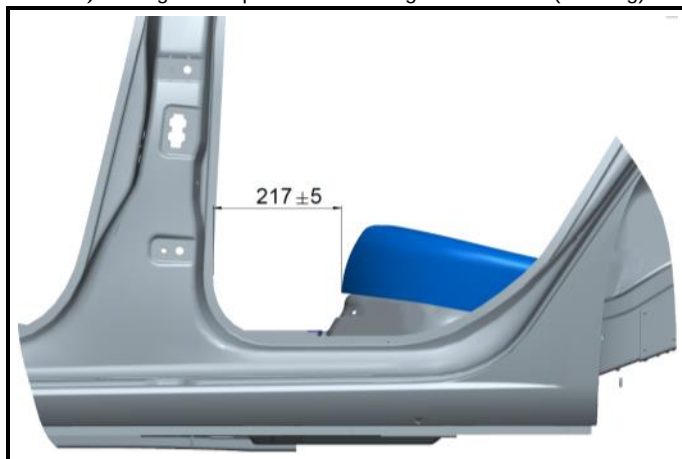
XII-A2) Longitudinal position of the original back seat (Drawing)
