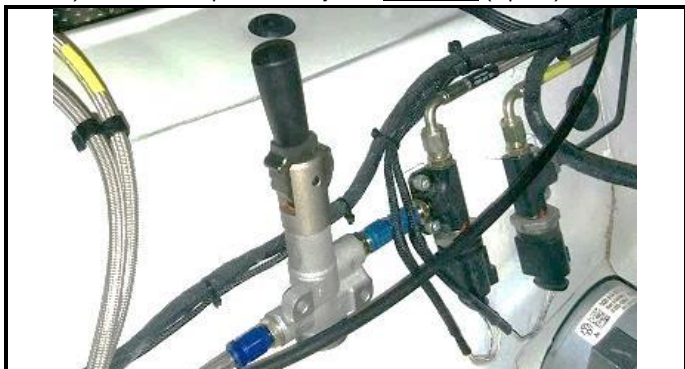
J11-5) Rear brake pressure adjuster in location (Option)
