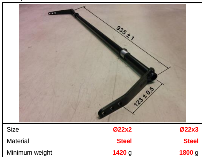
G7-1) Anti roll bar dismounted
