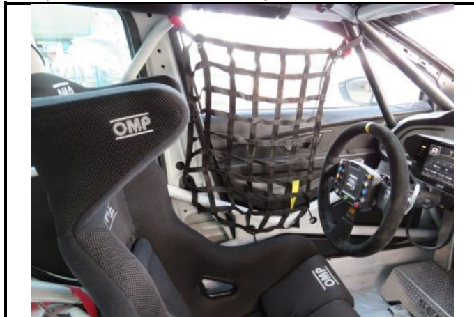
S5-2) Protective window net with fixings in location
