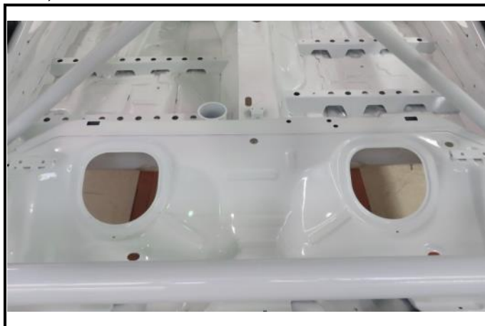
D1-6) Fuel sampling connector in location
