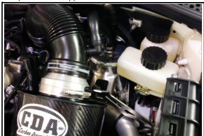
J8-1) Brake fluid tank(s) in location
