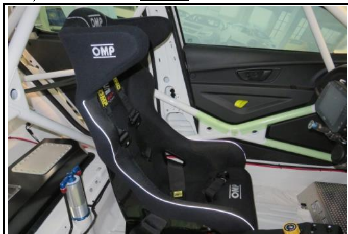
L2-5) Driver Seat installed in location
