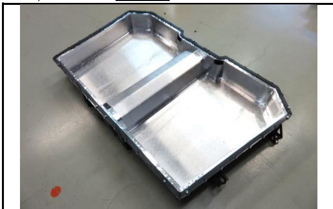
D1-23) Fuel tank vane dismounted
