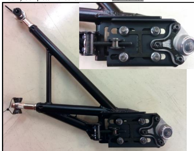
G5-2) Complete wishbone/arm front – dismounted
