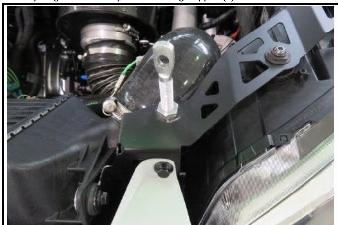
M5-1) Engine bonnet open - retaining support(s)
