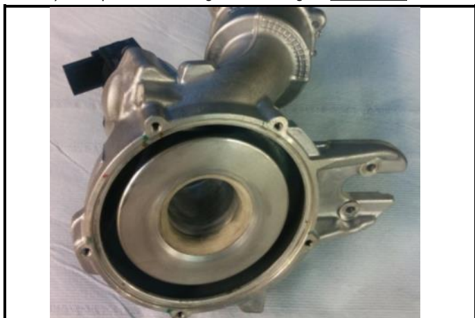
C15-7) Compression housing of turbocharger - dismounted
