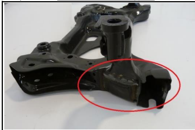
G2-6) Subframe – Supports' Modification
