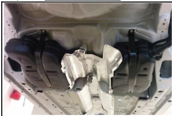
D1-4) Fuel tank filler cover and fire wall
