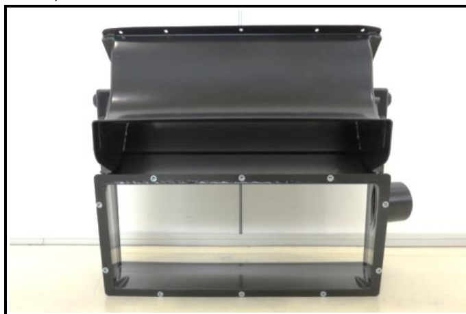
C13-6) Water cooler air ducts - dismounted
