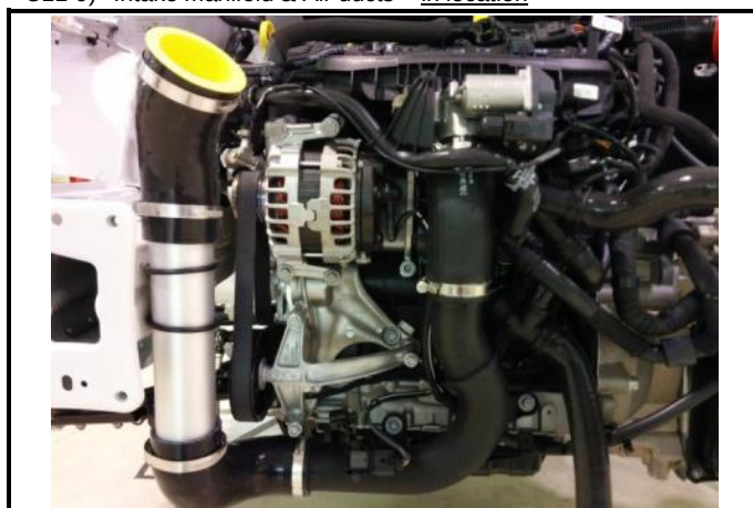
C11-9) Intake manifold & Air ducts – in location
