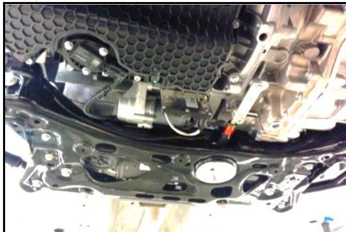
G2-2) Subframe in location
