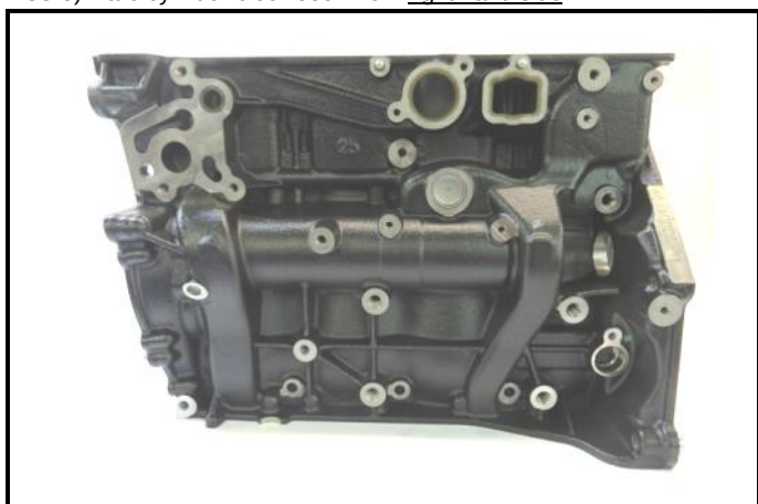
C3-3) Bare cylinder block seen from right hand side
