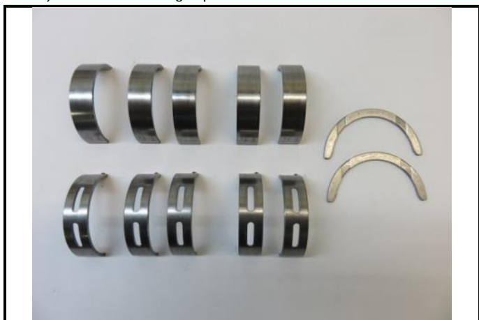
C3-7) Crankshaft bearing caps
