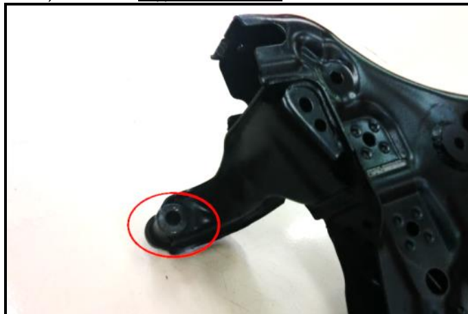
G2-6) Subframe – Supports' Modification
