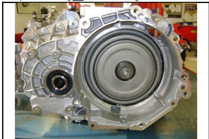
F2-1) Gearbox casing and clutch bell housing
