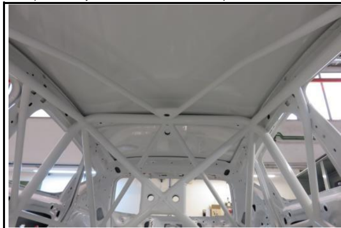
N1-6) Bare bodyshell – Roof seen from cockpit
