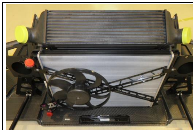
C13-2) Water radiator in location
