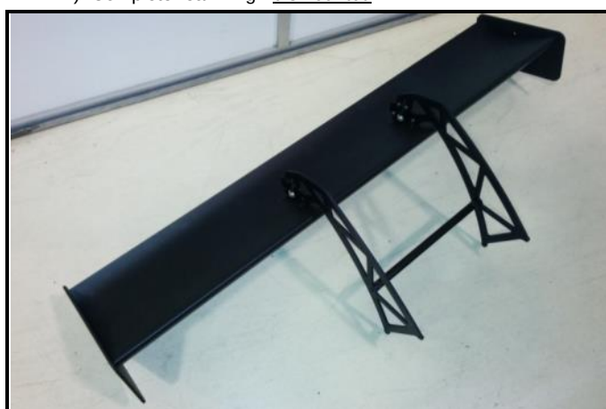
M14-2) Complete rear wing - dismounted
