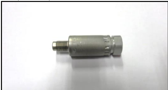
J11-3) Rear brake pressure valve in location (Option)
