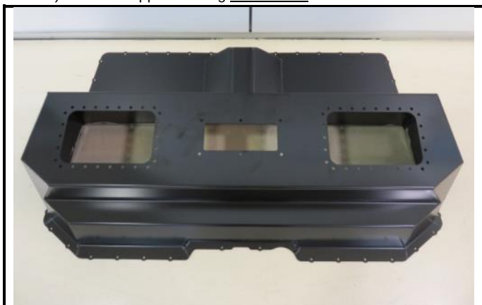
D1-21) Fuel tank upper housing dismounted
