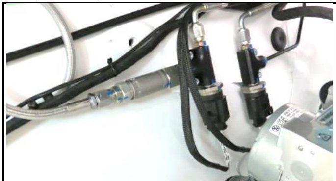
J11-5) Rear brake pressure adjuster in location (Option)
