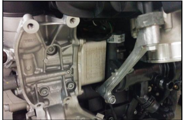
C14-10) Oil cooler – mounted in location
