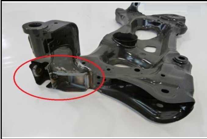
G2-5) Subframe – Modification of axle mounting points
