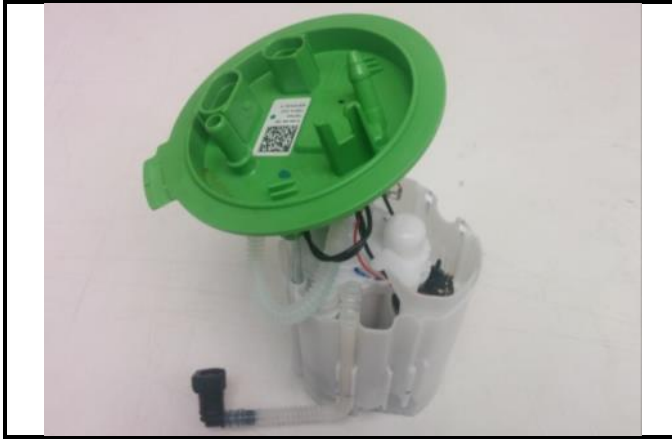
D1-7) Low pressure fuel pump(s) - dismounted
