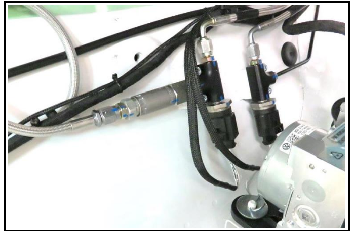
J11-4) Rear brake pressure adjuster in location (Option)
