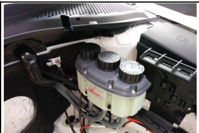
J8-1) Brake fluid tank(s) in location
