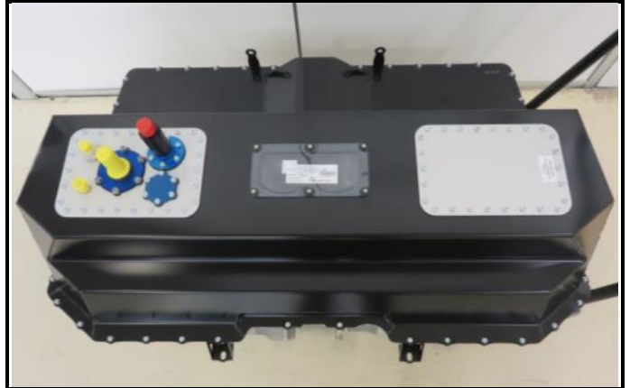
D1- 22) Fuel tank upper housing in location
