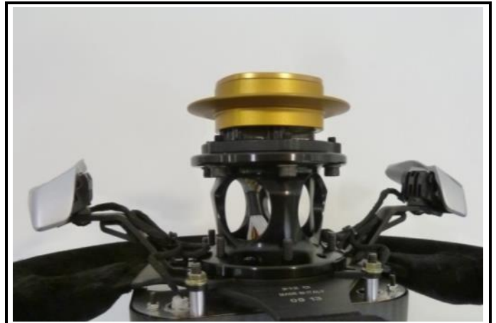
J12-2)Steering wheel release mechanism
