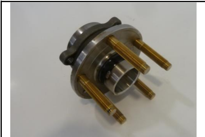
I1-3) Front wheel attachment dismantled
