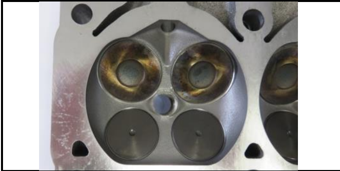
C8-7) Combustion chamber
