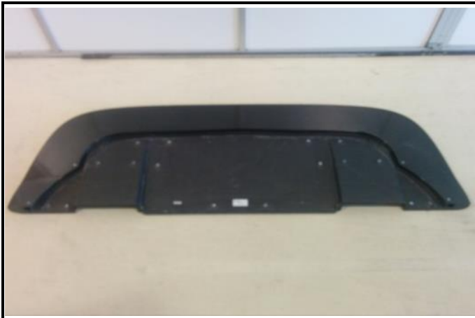
M15-3) Complete front splitter brackets – front view
