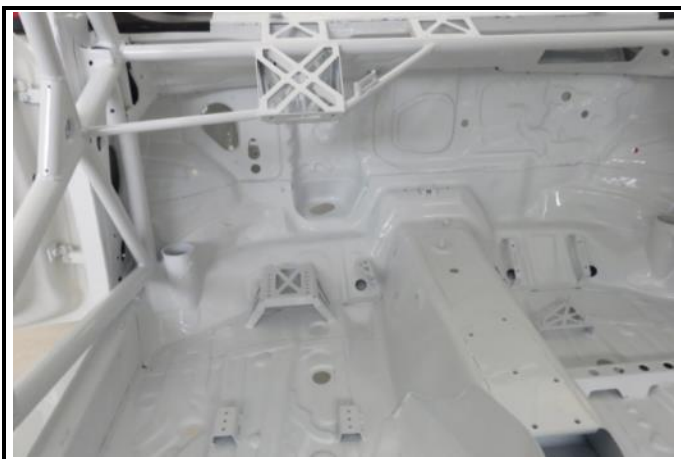
N2-1) Interior view on modifications for pedal box, steering column and air jacks
