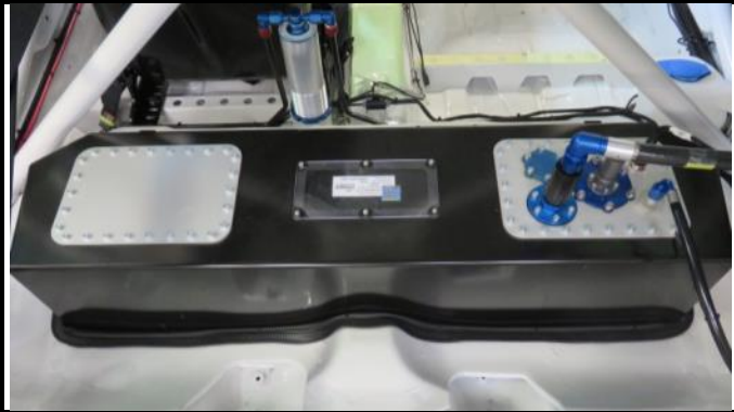
D1-17) Fuel tank in location (view on identification plate)
