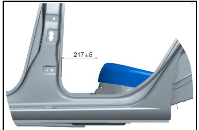
XII-A2) Longitudinal position of the original back seat (Drawing)
