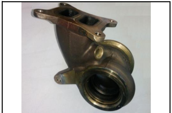
C15-8) Turbine housing of turbocharger - dismounted
