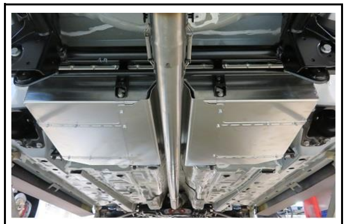
D1-16) Fuel tank in location (view from below)
