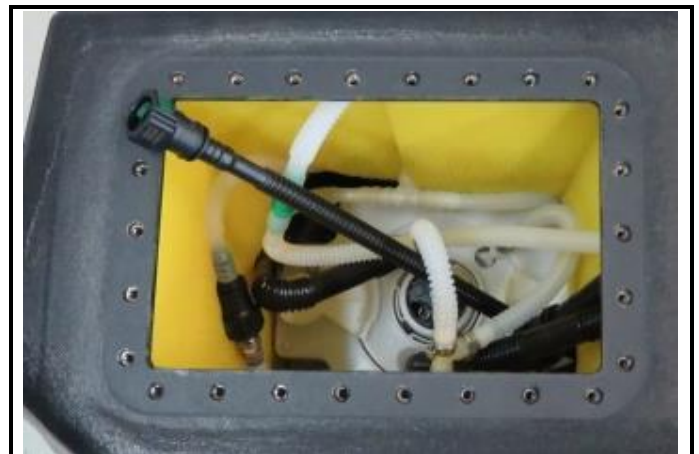
D2-4) Low pressure fuel pump - in location
