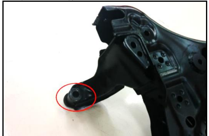
G2-6) Subframe – Supports' Modification
