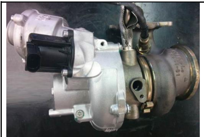
C15-1) Plan view of complete turbocharger unit
