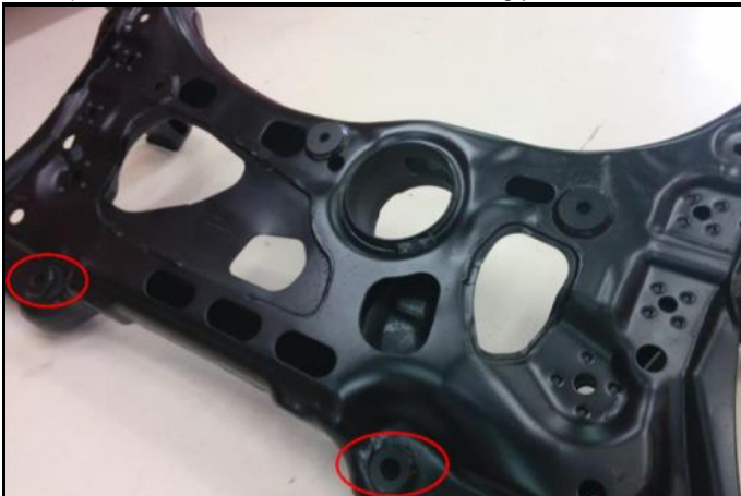
G2-5) Subframe – Modification of axle mounting points
