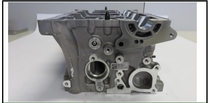
C8-6) Bare cylinder head seen from flywheel side
