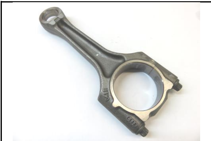
C5-1) Connecting rod from \frac{3}{4} on big end side
