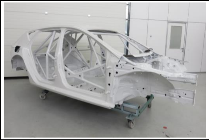
N1-3) Bare bodyshell – Engine compartment
