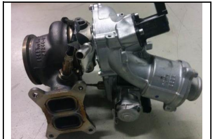
C15-2) Front view of complete turbocharger unit
