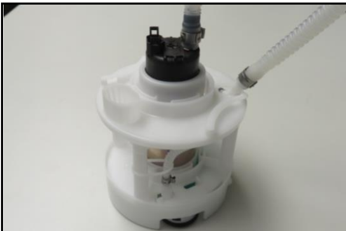
D2-3) Low pressure fuel pump - dismounted
