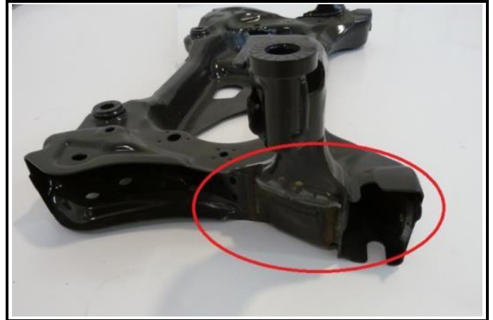
G2-6) Subframe – Supports' Modification
