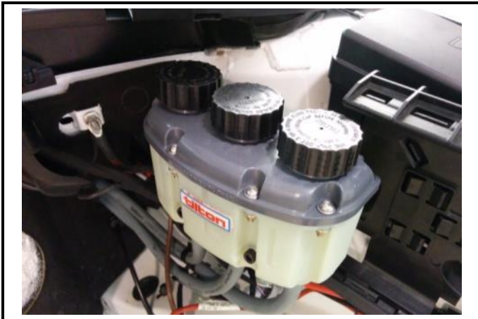
F1-5) Clutch fluid reservoir in location
