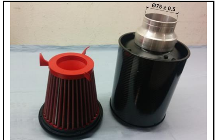
C11-2) Air filter and its housing - dismounted
