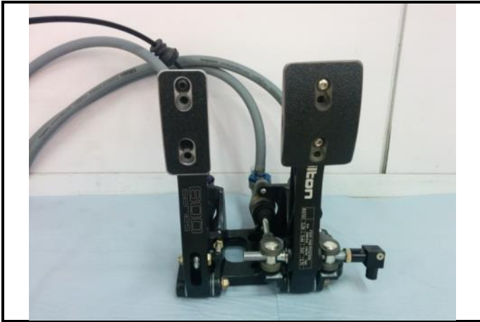
L2-3) Pedal box - mounted in location
