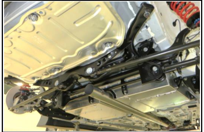
H2-2) Subframe in location
