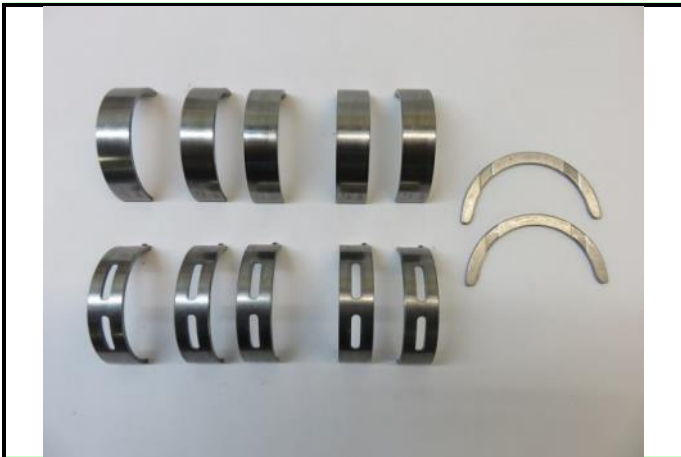
C3-7) Crankshaft bearing caps
