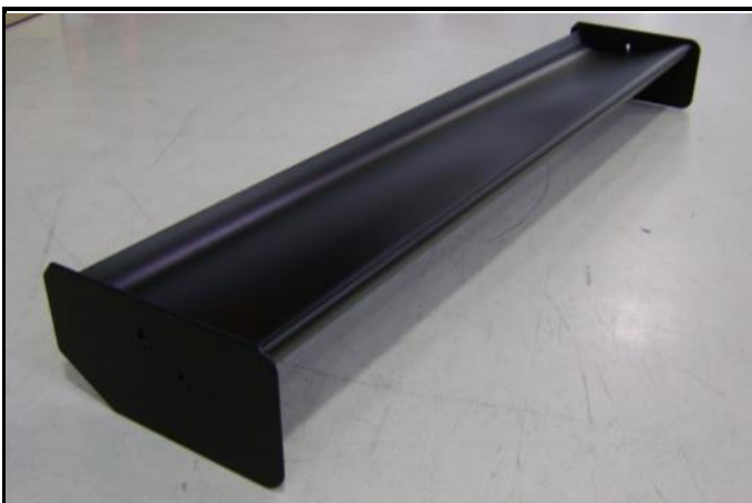
M14-1) Complete rear wing - dismounted
