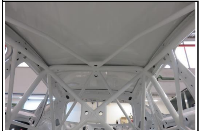
N1-6) Bare bodyshell – Roof seen from cockpit
