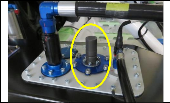
D1-21) Fuel tank upper housing dismounted
