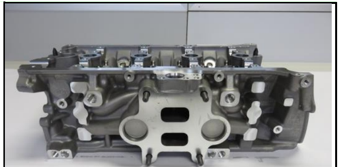
C8-6) Bare cylinder head seen from flywheel side
