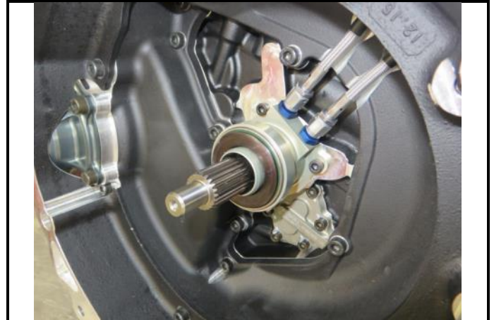
F1-4) Clutch release bearing in location
