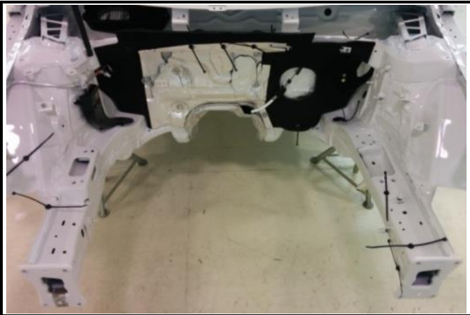
N1-5) Bare bodyshell – Cockpit seen from rear window opening
