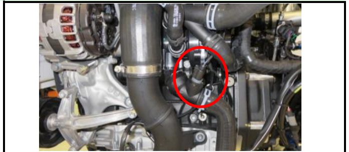
ENGINE WATER TEMPERATURE IN LOCATION
