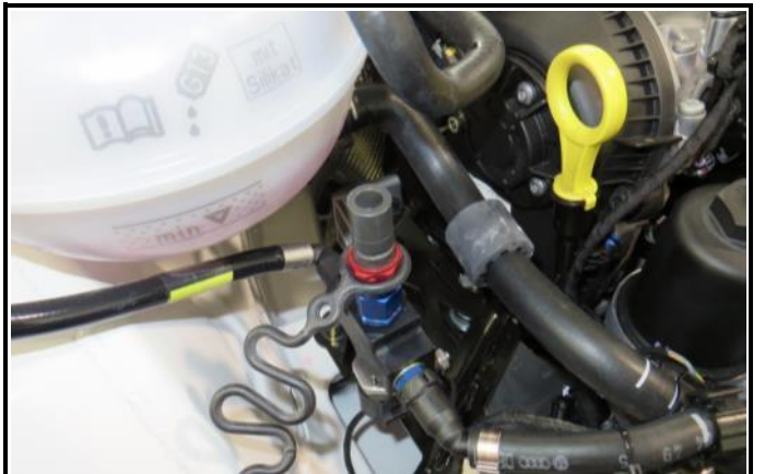
D1-6) Fuel sampling connector in location
