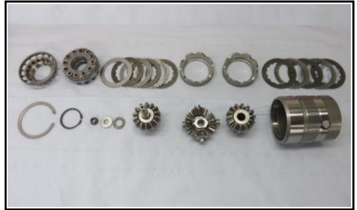
F4-6) Differential dismantled
