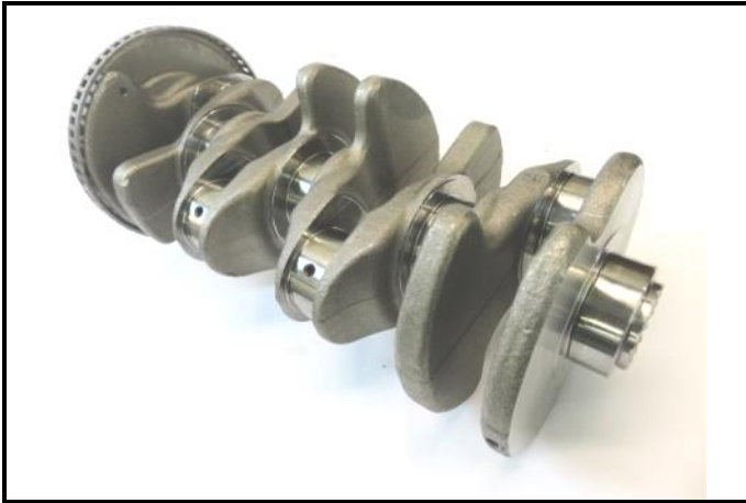
C6-3) Alternative crankshaft bearings
