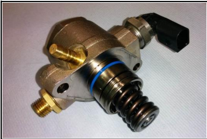
D2-3) Low pressure fuel pump - dismounted
