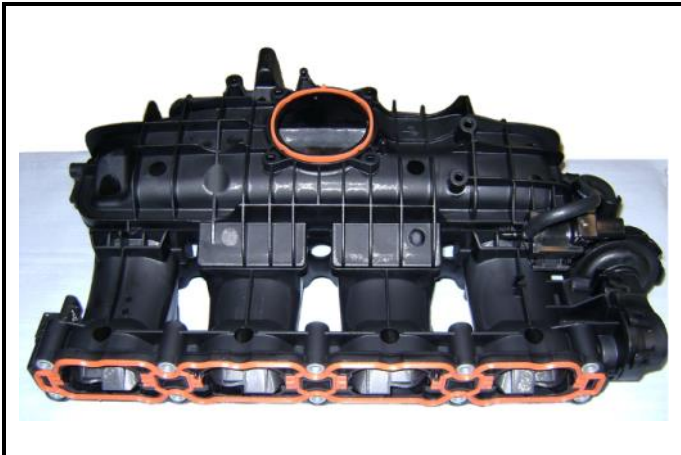
C11-1) Intake manifold - dismounted
