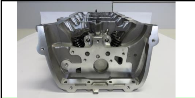
C8-5) Bare cylinder head seen from timing side
