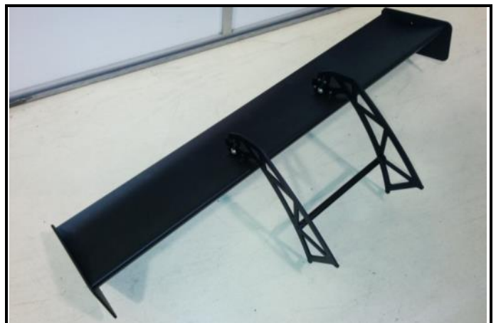
M14-2) Complete rear wing - dismounted
