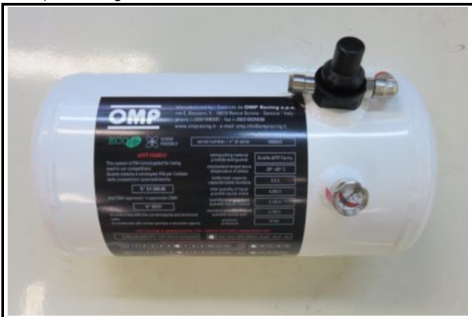
S4-1) Fire extinguisher dismantled
